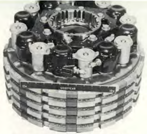
One of eight new carbon brake stocks used on the B-1. Combined weight of all stocks is only 512 lbs.
