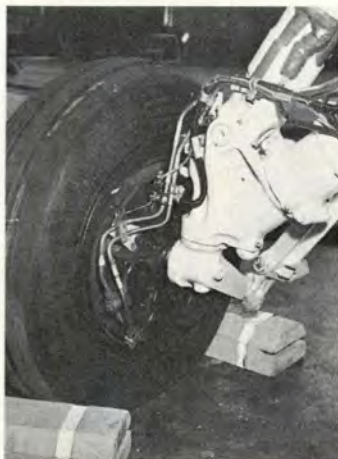
Lightweight carbon brake installation on the F16. New fibers added to the carbon discs have allowed smaller size and retention of braking power when water soaked.
